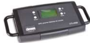
CTL3520 handheld GPS jamming detector with direction finding capability
